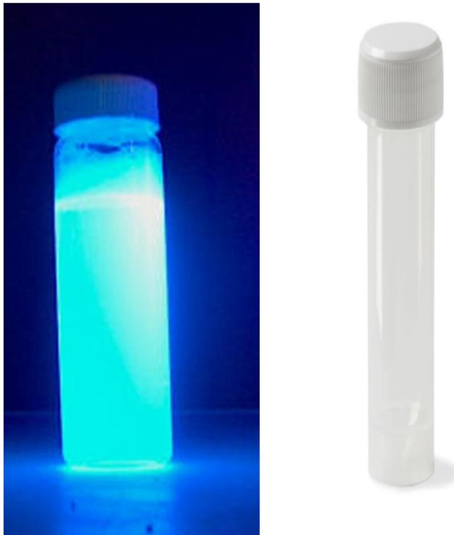
Left: A tube with optical brighteners exposed with UV light.
